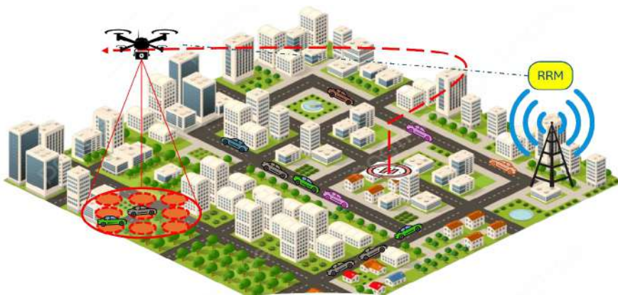
A UABS moves in a urban environment and cooperates with the terrestrial base station to provide service to vehicular users.
